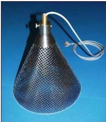
Fig. 9. The Conical metal housing for the CFL.
