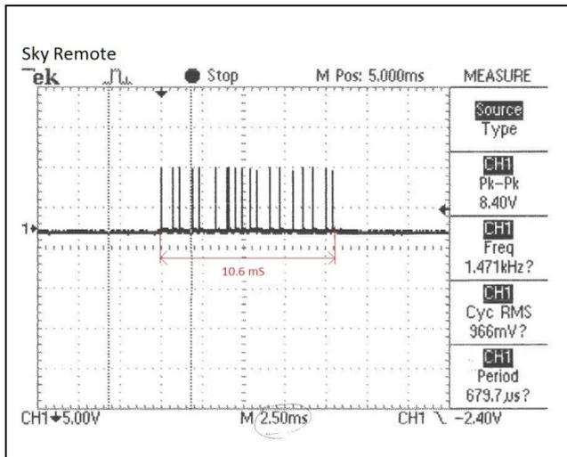
Fig. 5. Measured pulses from Infrared Remote controller.
