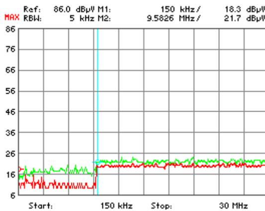
Fig. 14. Green – LISN connected to normal mains, Red – LISN connected to generator.
