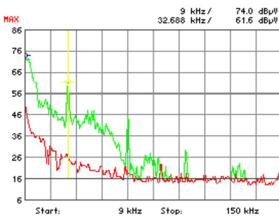
Fig. 13. Green – LISN connected to normal mains, Red – LISN connected to generator.
