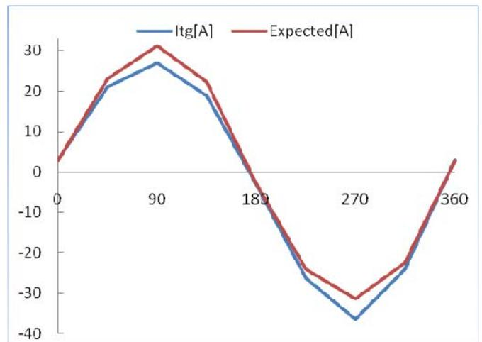
Fig. 8. Measured Inrush current when multiple CFLs are switched ON.
