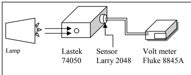
Fig. 2. Experimental setup 1.
