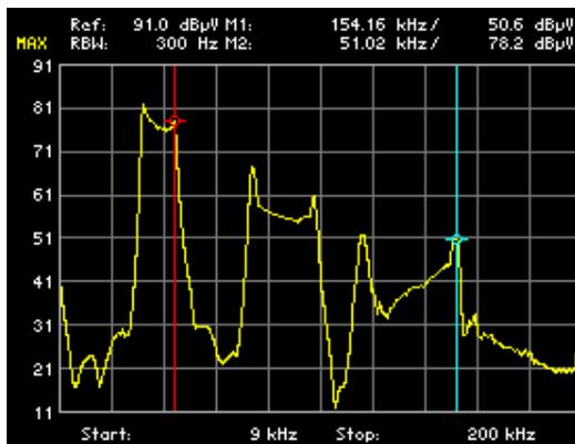
Fig. 15. Ecobulb spectrum in 9 kHz to 200 kHz range.
