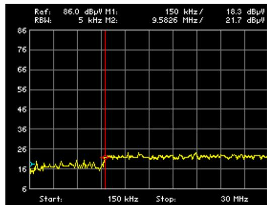
Fig. 12. Spectrum of 150 kHz - 30MHz; light turned off.
