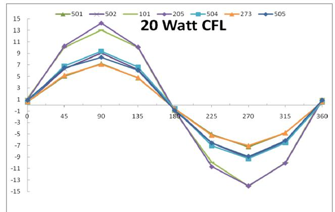
Fig. 7. Inrush Current as a Function of Turn-On time for various 20W CFL models.
