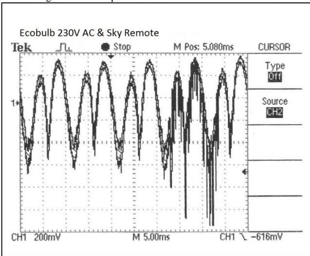
Fig. 6. Measured Infrared with Ecobulb.
