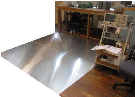
Fig. 10 Test Setup: the ground plane, lamp holder and Spectrum analyser.
