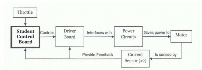
Figure 5 Go-cart drive block diagram
