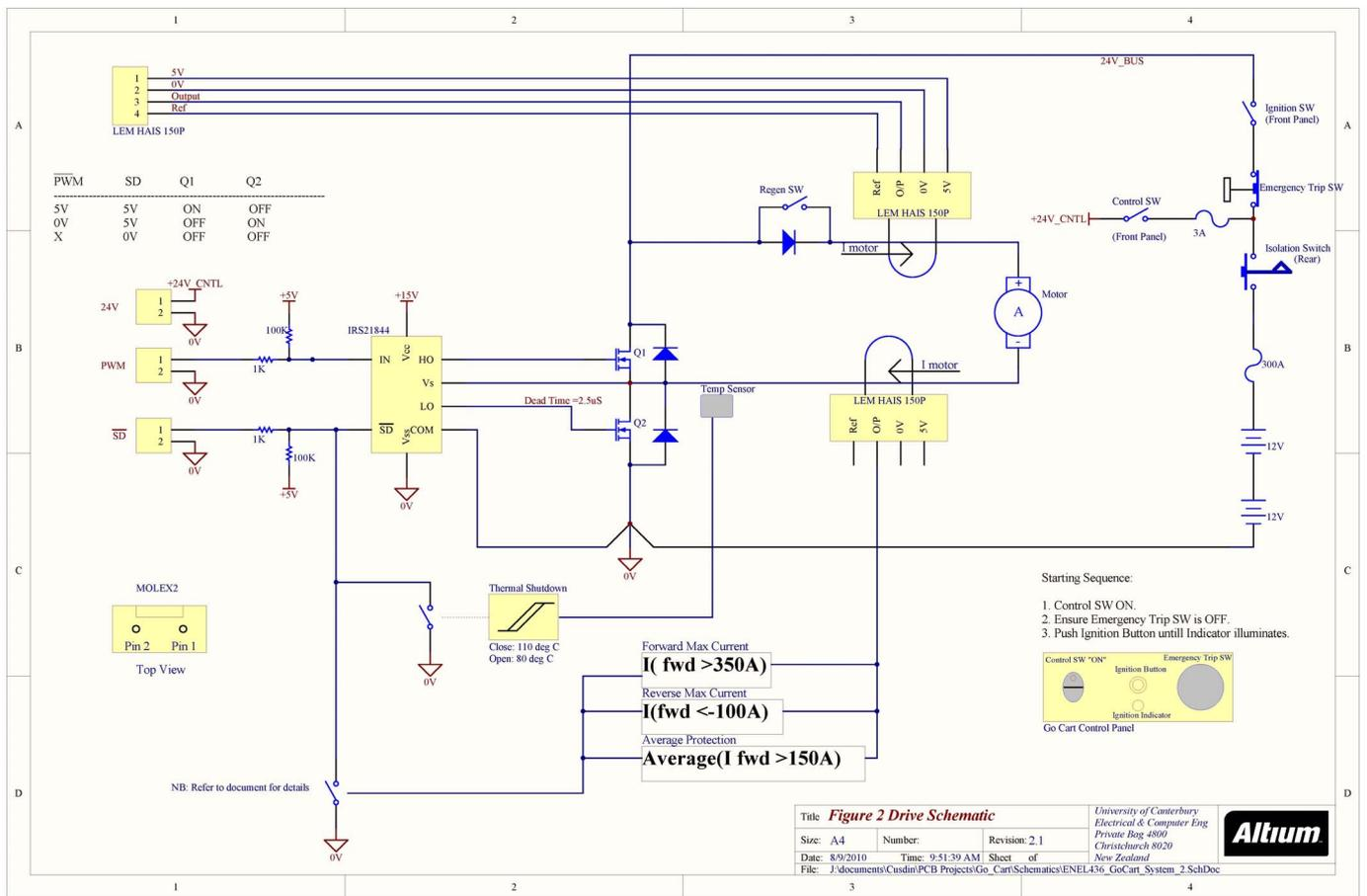
Figure 2 Go-cart drive schematic
