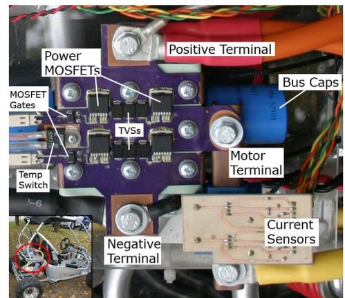
Figure 3 Power circuits
