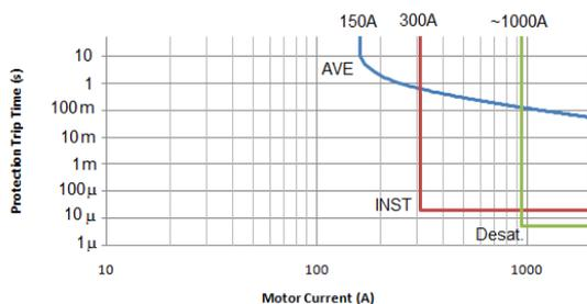
Figure 4 Forward current protection coordination
