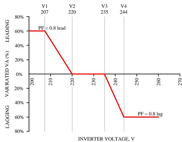
Curve for the NZ inverter Volt-VAR response mode designed by EPECentre/Network Analysis Group
